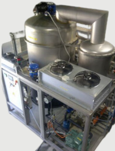
Evaporator used in the hazardous waste treatment process at Le Mans, France.
